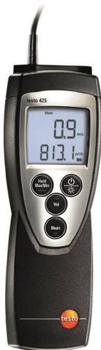
It is instrumental toward the air flow speed in chamber – according the standart. The speed is measured by this way – the anemometer is before the test intromit to chamber the upper part ( to socket). During the test is anomometer pushed out and the measuring is not made.
