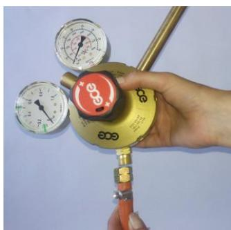
The operator moves the torch away from the sample and removes the adapter (stop). Connects the hose to the pressure reducing valve. It releases the gas and checks the gas pressure setting at 10 to 50 kPa.
