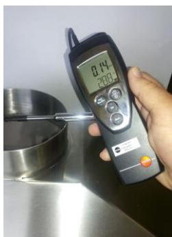
He closes the door, places the anemometer sensor in the middle of the chimney and sets the flow velocity to  $0.7 \pm 0.1$  m / s by using the extractor hood.
